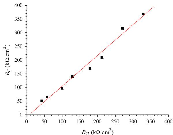
**Fig. 9.** Graphical juxtaposition of the values of the polarisation resistance  $R_p$  acquired by polarisation measurements (Table 2a) with the values charge transfer resistance  $R_{ct}$  estimated by the impedance spectra (Table 4).
