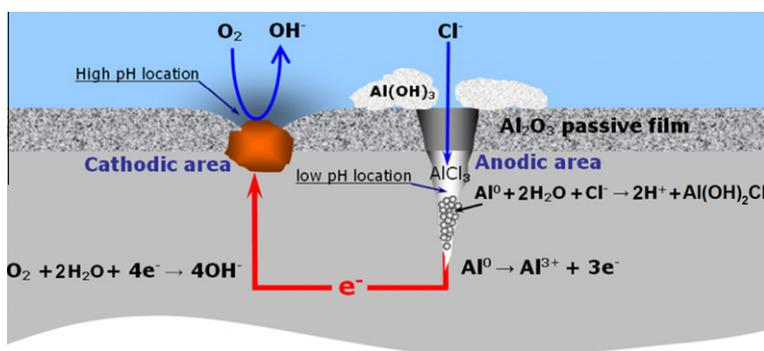
Fig. 5. An illustrative model of acidic pitting formation in the case of AA2024 aluminium alloy corrosion.
