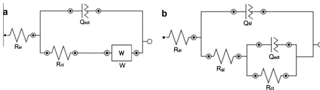
Fig. 8. Equivalent circuits used for structural impedance modelling.  $R_{el}$  – electrolyte resistance;  $R_{ct}$  – charge transfer resistance;  $R_{sl}$  – resistance of the superficial salt layer;  $Q_{edl}$  – constant phase element of the double electric layer;  $Q_{sl}$  – constant phase element of the superficial salt film and  $W$  – Warburg element.
