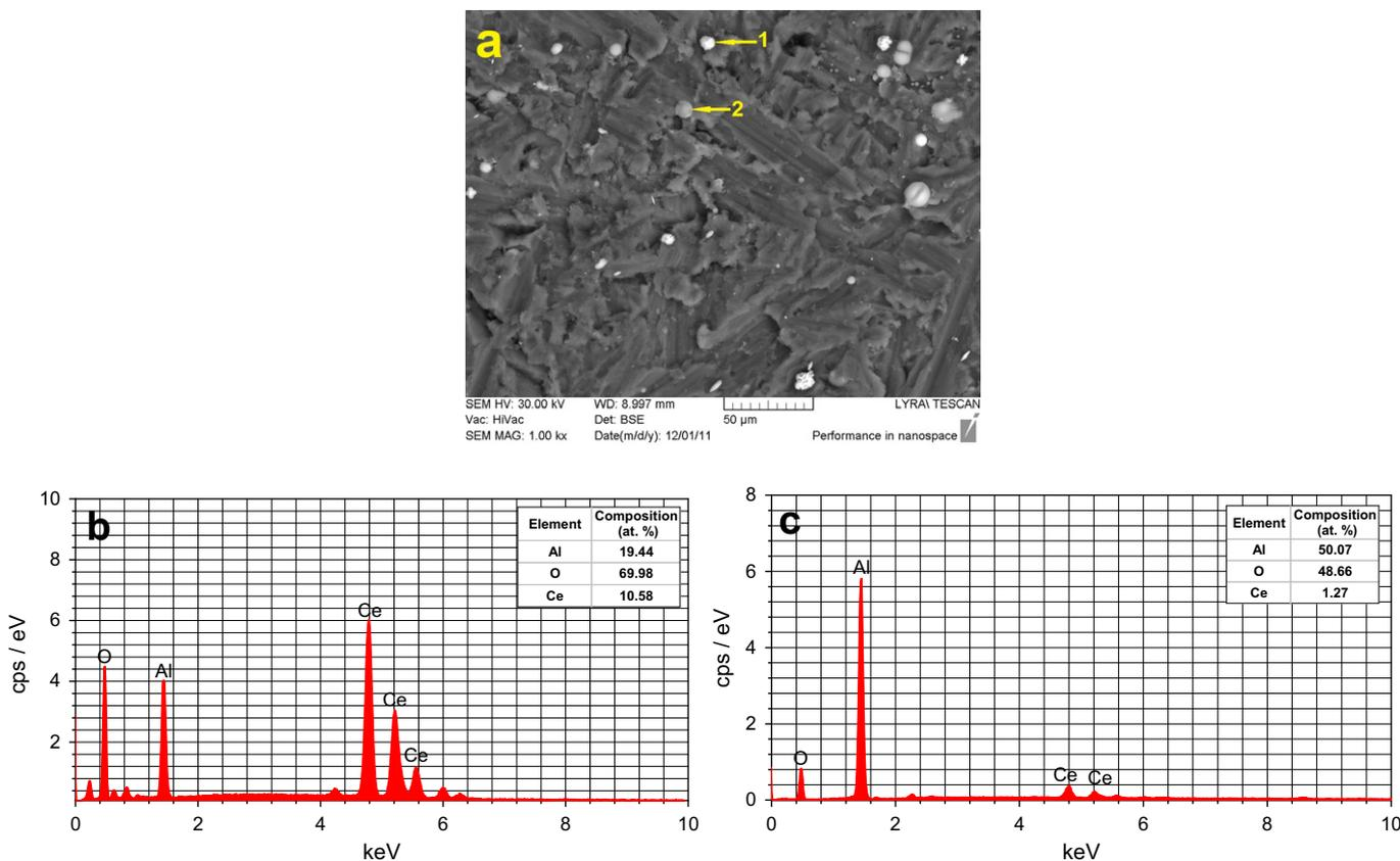
Fig. 4. SEM image (a) and EDS spectra (b and c) of AA2024 specimen, after 600 h of exposition to 0.01 M NaCl solution, with  $1 \times 10^{-3}$  M concentration of  $\text{Ce}(\text{NO}_3)_3$ .
