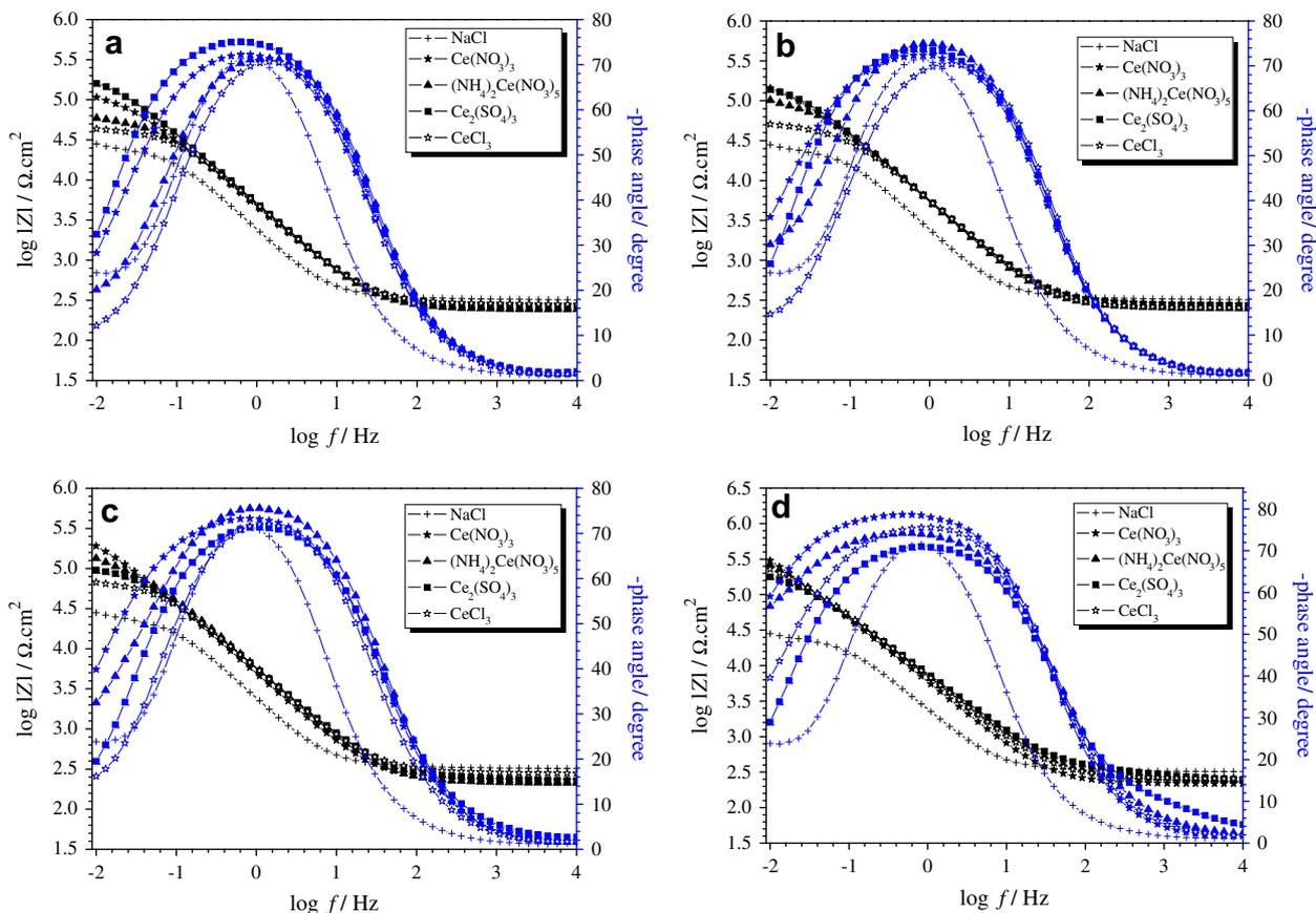
Fig. 7. Impedance spectra in Bode plots for samples of the alloy for different times of exposure to model corrosive media, composed by 0.01 M NaCl with  $1 \times 10^{-3}$  M concentration of the respective Ce salts: (a) 24 h; (b) 72 h; (c) 144 h; (d) 600 h.
