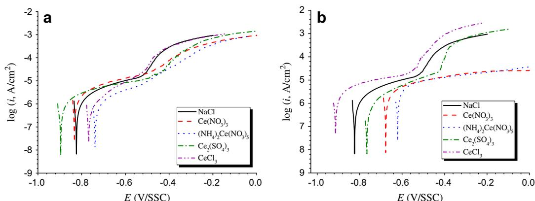
**Fig. 3.** Anodic polarisation curves of AA2024 specimens, after 24 h of exposure into 0.01 M NaCl solutions without and with (a)  $5 \times 10^{-5}$  M and (b)  $1 \times 10^{-2}$  M concentration of the respective Ce(III) salts.
