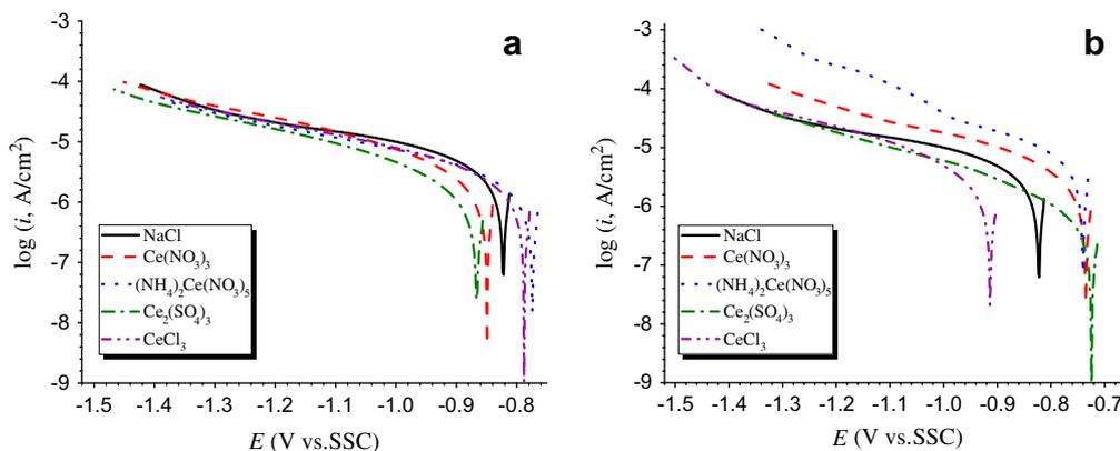
Fig. 2. Cathodic polarisation curves of AA2024 specimens after 24 h of exposure into 0.01 M NaCl solutions without and with: (a)  $5 \times 10^{-5}$  M and (b)  $1 \times 10^{-2}$  M concentration of the respective Ce(III) salts.
