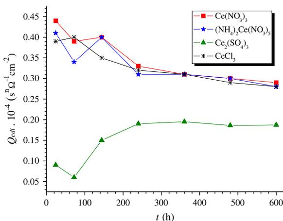
**Fig. 11.** Evolution of the electric double layer capacitance in metal/electrolyte interface within the exposure time of the specimens into the model corrosive media with  $1 \times 10^{-3}$  M concentration of different cerium salts.
