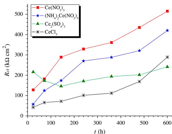
**Fig. 10.** Development of the charge transfer resistance within the exposure time of the specimens into the model corrosive media with  $1 \times 10^{-3}$  M concentration of different cerium salts.
