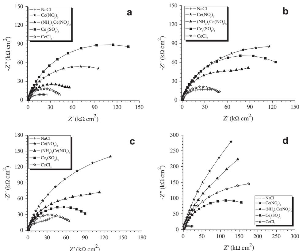
**Fig. 6.** Impedance spectra in Nyquist plots for samples of the alloy for different times of exposure to model corrosive media, composed by 0.01 M NaCl with  $1 \times 10^{-3}$  M concentration of the respective Ce salts: a – 24 h; b – 72 h; c – 144 h; d – 600 h.
