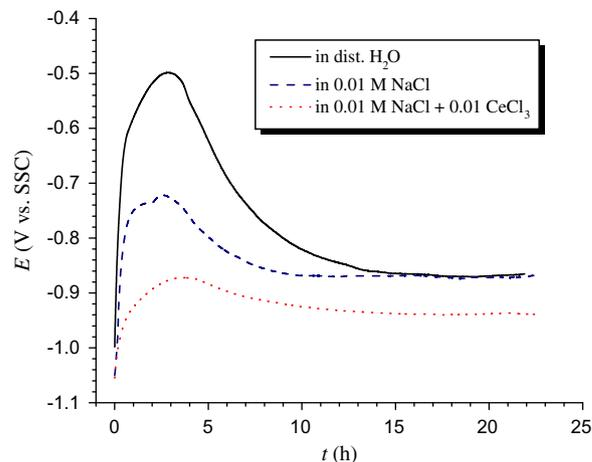
**Fig. 1.** Evolution of  $OCP$  within the exposition time for AA2024 samples immersed in different media.
