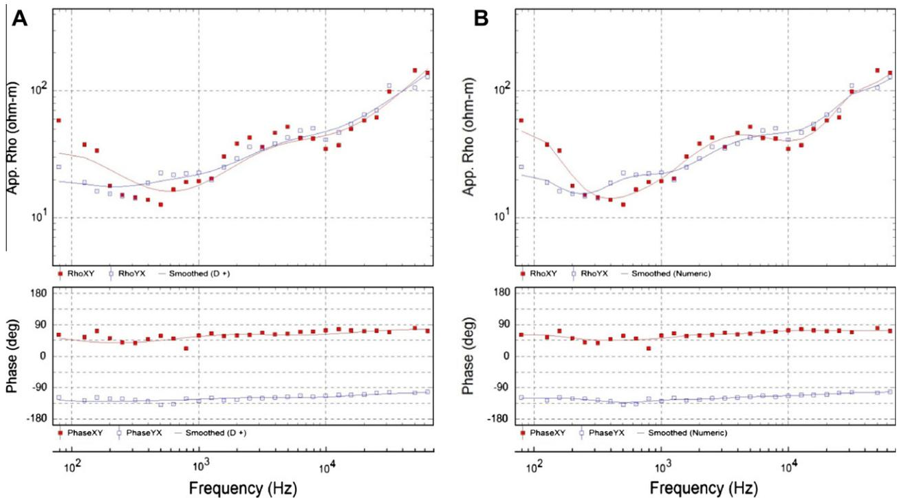
Fig. 4. Comparison of the smoothed curves generated from the two different smoothing methods on station S2. The smoothed curve in (A) is generated by the D+ algorithm whereas that of (B) is achieved through the numerical method.
