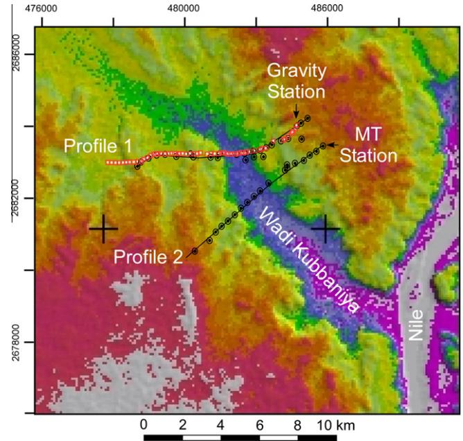
Fig. 3. Digital Elevation Model (DEM) of the study area showing the location of the MT and gravity data collected across Wadi Kubbania. The MT data were collected at a 250 m station spacing whereas the gravity data were collected at 100 m spacing. Poor contact or harsh terrain required some stations to be offset or moved closer to one another.
