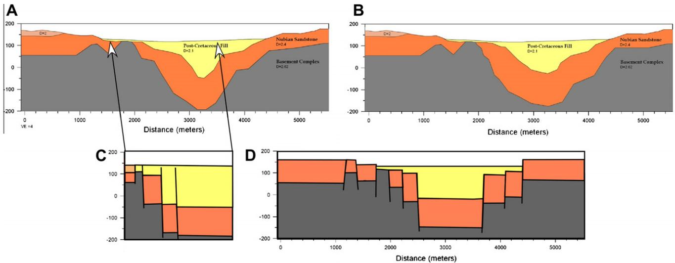
**Fig. 8.** (A) and (B) gravity models structured around D+ and numerically smoothed MT data, respectively. (C) Subsurface model of the western half of Wadi Kubbaniya from seismic refraction data. Modified after Atef (2011). (D) Conceptual model illustrating the Wadi Kubbaniya as a graben filled with post-Cretaceous sedimentary rocks.
