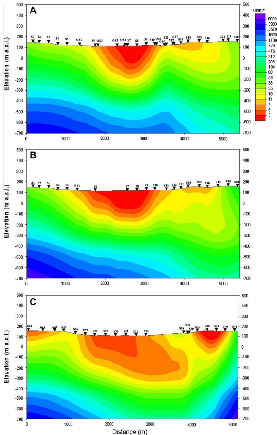
**Fig. 5.** Two-dimensional (2D) inversion of station soundings from Profile 1 smoothed using the D+ algorithm (A) and numerically smoothed (B). (C) 2D Inversion of station soundings from profile 2 smoothed with the D+ algorithm.
